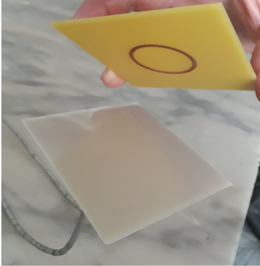
Figure 4.5.4: Multilayer Ring resonator in measurement test (Mylar-A).
