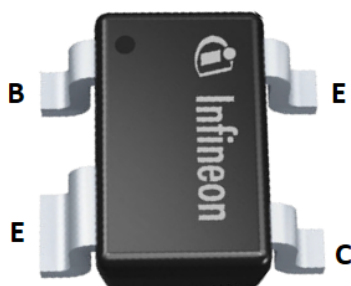
Figure 7.4.1: Pinout of the transistor Infineon BFP720: B = base, C = collector, E = emitter.
