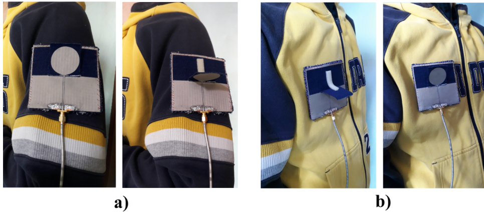
Figure 2.2.26: On-body measurement set-up for both antenna topologies: a) antenna on an arm; b) antenna on the chest.
