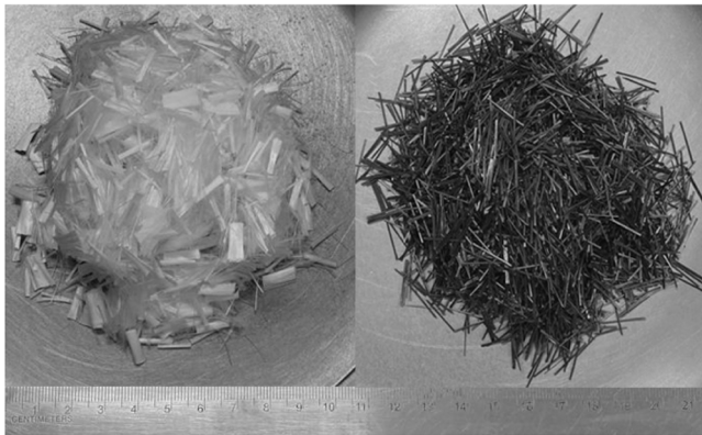
Fig. 2. (left) Glass fibers; (right) Basalt fibers.
