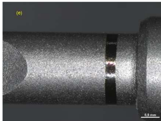
Figure 6. Photos of pilot drill no. 3 obtained under the microscope before use. Photos of pilot drill no. 2 obtained under the microscope before use. (a) Image of the drill at tip level, (b–d) images of the drill in the middle, (e) image of the drill at the end part.
