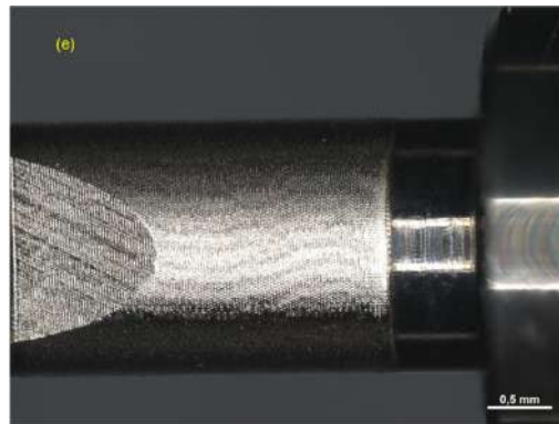
Figure 16. Photos obtained under the microscope of pilot drill no. 2 (a) after use and sterilization cycles at tip level (b), in the middle (c,d), and at the end part (e).
