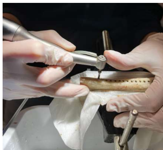
Figure 13. A lance cutter drilled 15 holes on each rib, spaced \geq 3 mm apart, totaling 45 holes across three ribs. Each sample used a different pilot drill.
