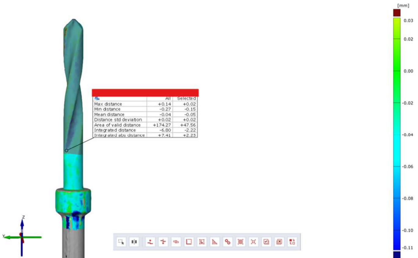
Figure 23. Surface comparison shows a maximum thickness increase of +0.02 mm, a minimum reduction of −0.15 mm, and an average deformation of −0.05 mm across the analyzed surface.
