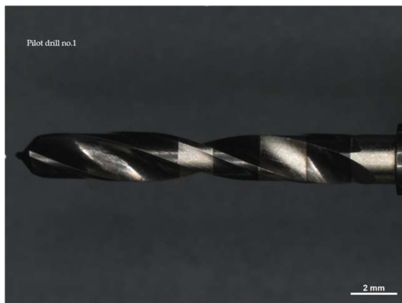
Figure 1. Drill no. 1 is an autoclavable stainless steel drill with a diameter of 2.2 mm. It operates at a maximum speed of 800 rpm with irrigation.
