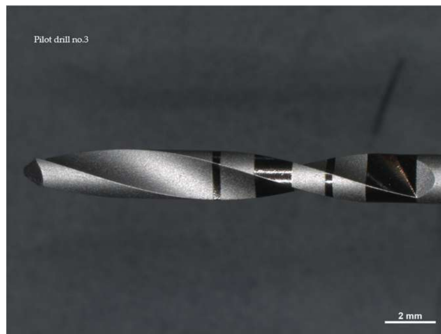
Figure 3. Drill no. 3 is constructed from stainless surgical steel and has a diameter of 2 mm.
