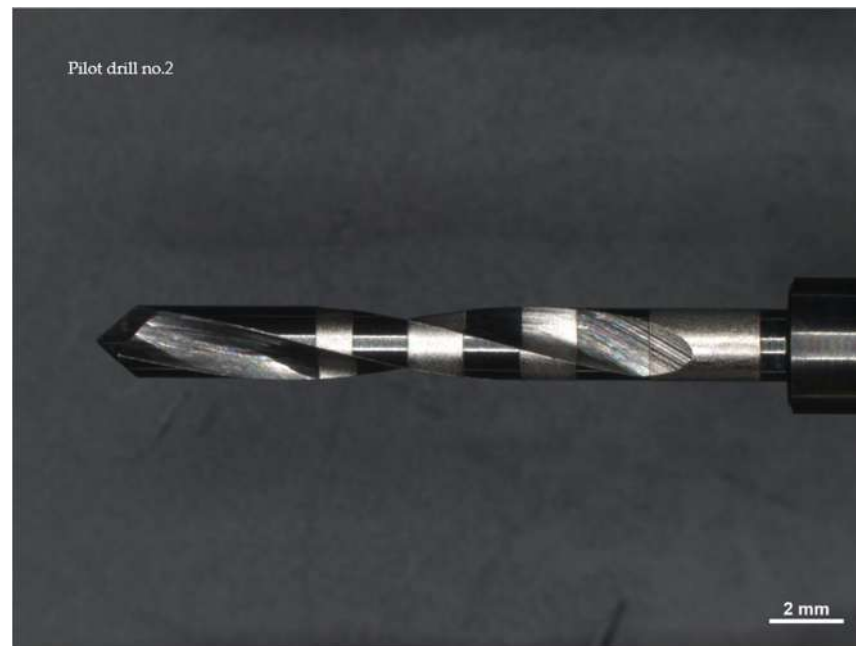
Figure 2. Drill no. 2 is a cylindrical cutter with a diameter of 2 mm, made of carbide-coated stainless steel. Recommended cutting speed: 900–1100 rpm.
