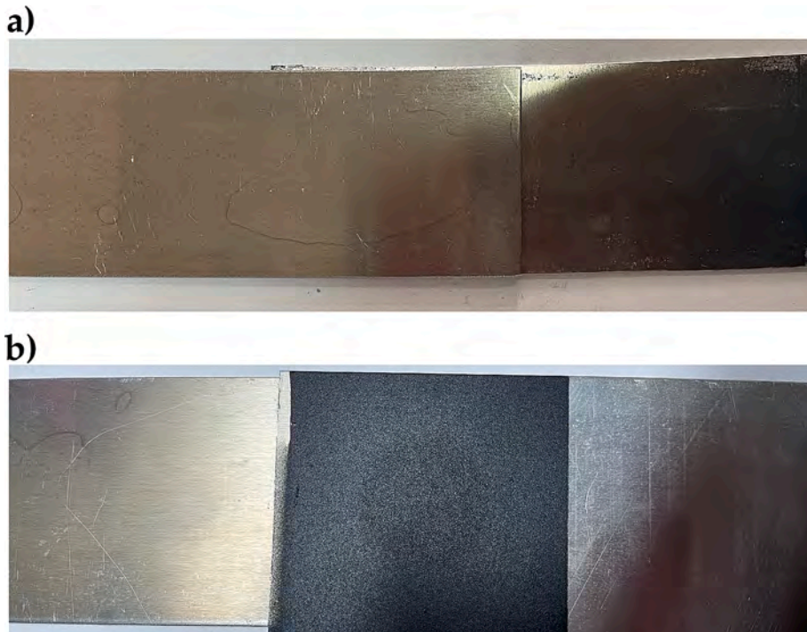
Fig. 4. (a) Two overlapped plates adopted as reference specimen for the non-welded behaviour. (b) Detail of inspected coated surface of welded specimen before the tensile-shear test.
