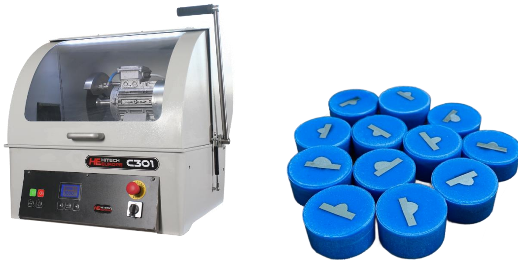
Figure 55. a). HITECH C301 cutting machine, b) englobed samples
