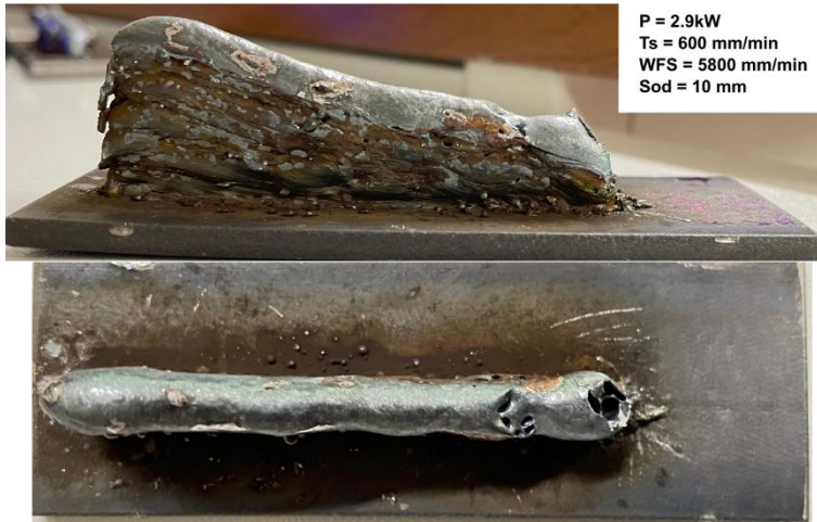
Figure 79. Humping effect in WAAM sample
