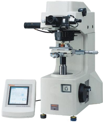
Figure 58 Mitutoyo HM-112 digital Vicker microhardness testing machine
