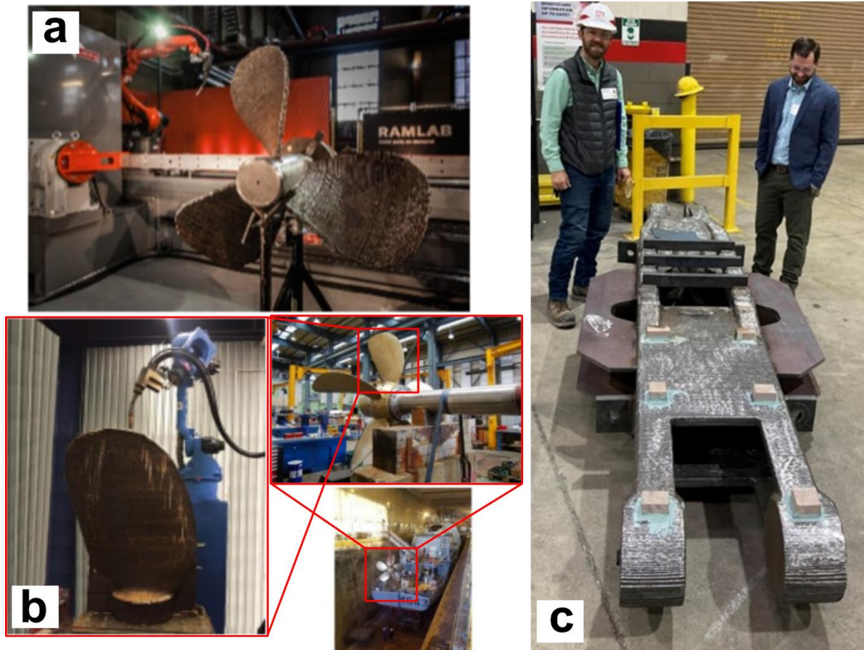
Figure 29. WAAM marine applications, a). marine propeller[137], b). spare part propeller blade [140], c). Poe Lock's ship arrestor system [138].
