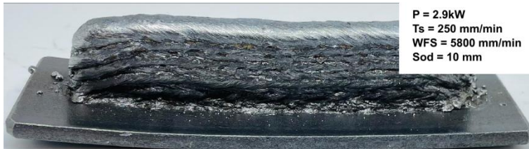
Figure 80. Bi-directionally deposited sample
