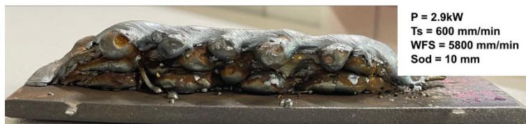
Figure 77 Without forced air-cooling.
