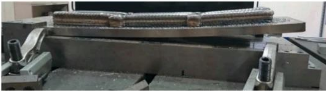
Figure 21. Distortion in WAAM produced parts [99].
