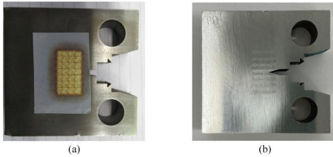
Figure 35. Laser shock peening on a sample a). during the process, b). after the process [168]
