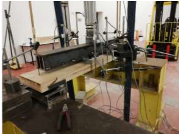
Figure 7. Short supply beech CLT panel under out plane load [59]
