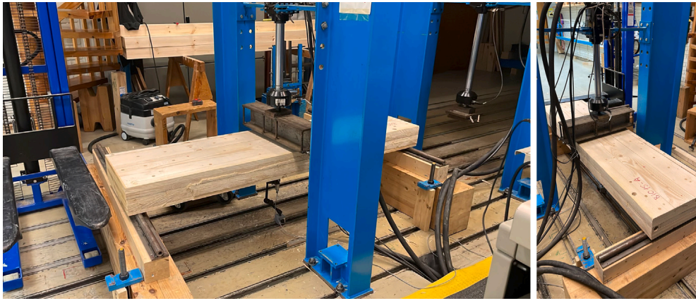
Fig. 4. Views of the experimental setup of the three-point bending test.
