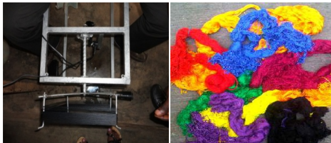
Figure 3. Mechanical skeiner used to convert yarns into hanks.
