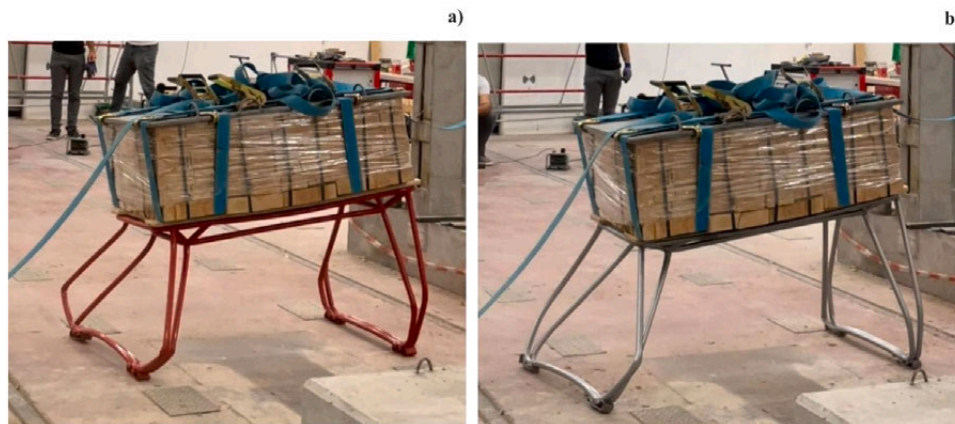
Fig. 17. Impact test performed with a brick stack of 450 kg: a) impact moment on V prototype; b) impact moment on S prototype.
