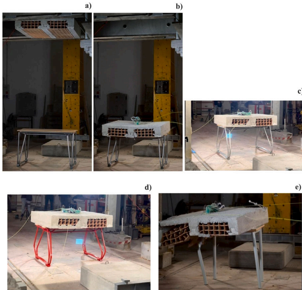
Fig. 18. Impact test performed with a floor portion of 300 kg: a) test setup prior to release; b) impact moment on S prototype; c) after the impact moment on S prototype; d) after the impact moment on V prototype; e) after the impact moment on traditional desk.
