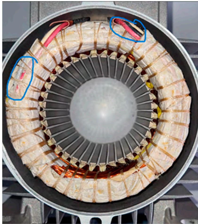
Figure 20. The stator of an induction motor after a fall from a height of 1 m.
