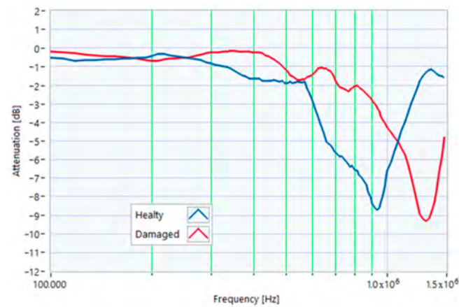
Figure 33. Comparison between TFs of the same motor in healthy conditions and with a shortcut between 2 winding turns.
