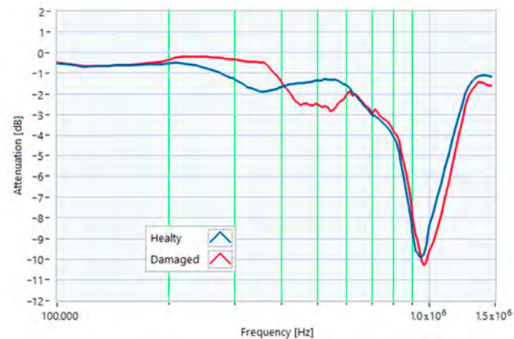
Figure 13. Comparison between TFs of the same motor in healthy conditions and with a 25 k \Omega resistance between one terminal and the ground.
