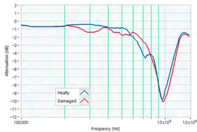
Figure 16. Comparison between TFs of the same motor in healthy conditions and with slight rotor misalignment.
