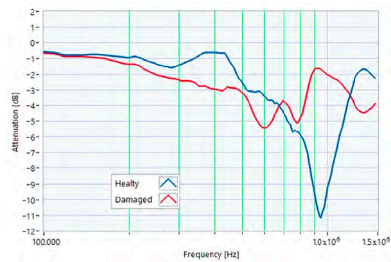
Figure 21. Comparison between TFs of the same motor in healthy condition and a stator fell from a height of 1 m.
