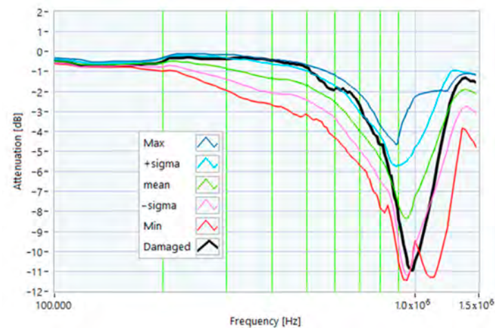
Figure 12. Comparison of the TF of a motor with a 1 \Omega resistance-in-series on a phase conductor with the reference TFs on the whole bandwidth.
