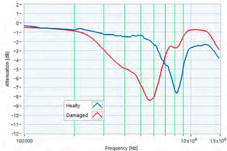
Figure 26. Comparison between TFs of the same motor in healthy conditions and with rotor bar damage.
