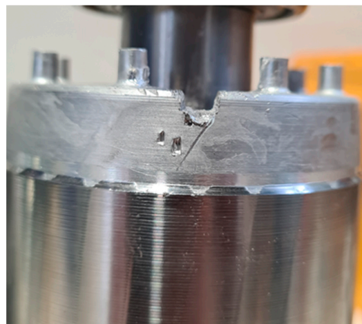
Figure 23. Shorting ring damage.
