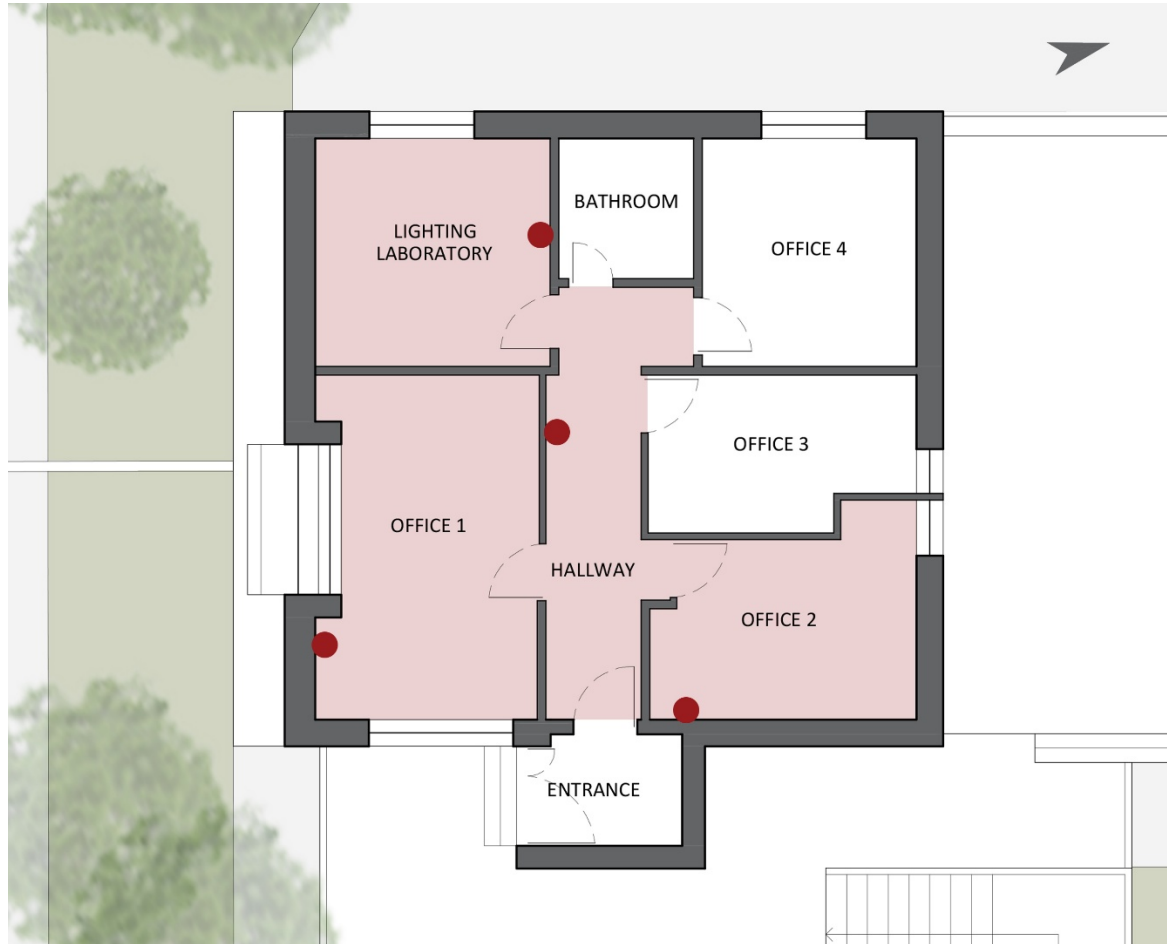
Figure 19. Areas affected by monitoring and indication of sensor nodes placement (red dots).
