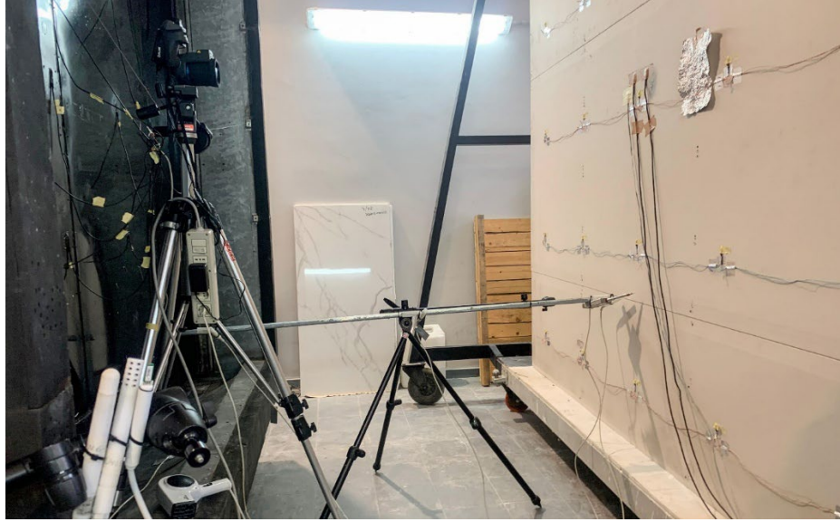
Figure 4. Experimental setup for the application of the M2 method. Cold side view.
