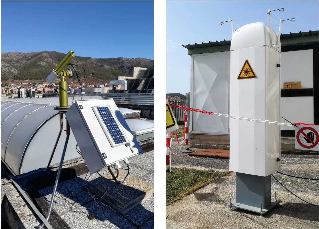
Figure 2.1: Instruments at LAO which are used in this work, notably the photometer CimeL CE318-TP9 (left) and the ceilometer Vaisala CL51 (right).
