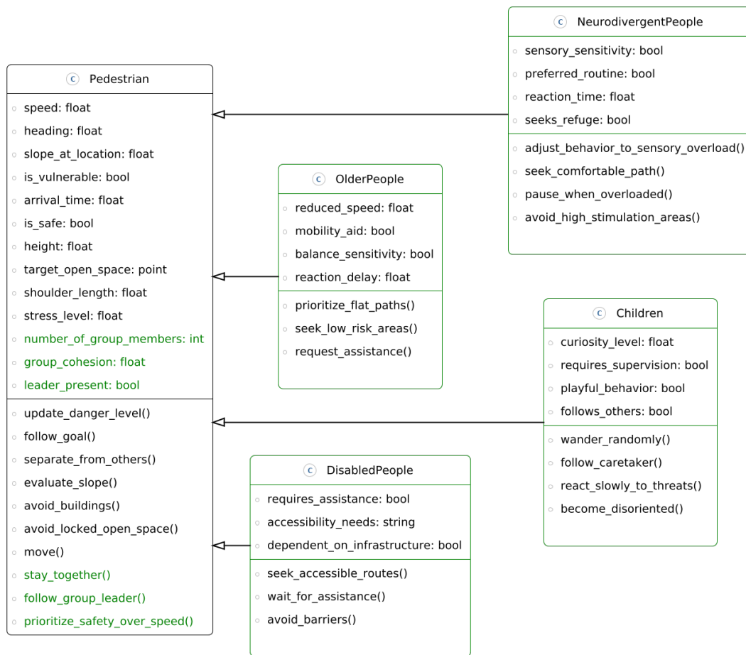
FIGURE 6.2: UML of Pedestrian specializations. Colored features mark deviations from Iskandar et al. [13]; green borders denote added classes.
