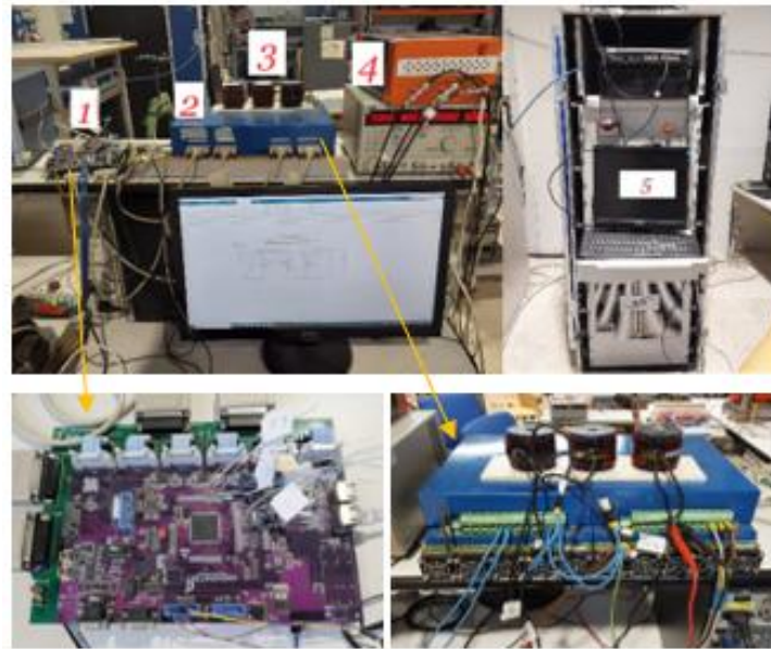
Figure 5.28: Experimental setup: 1) Control board, 2) Converter, 3) Input filter, 4) Grid voltages transducers, 5) Grid simulator.
