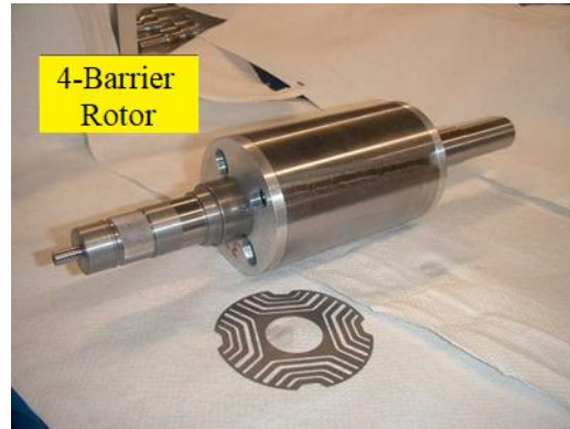
Figure 3.12a: SynRM utilized for the tests
