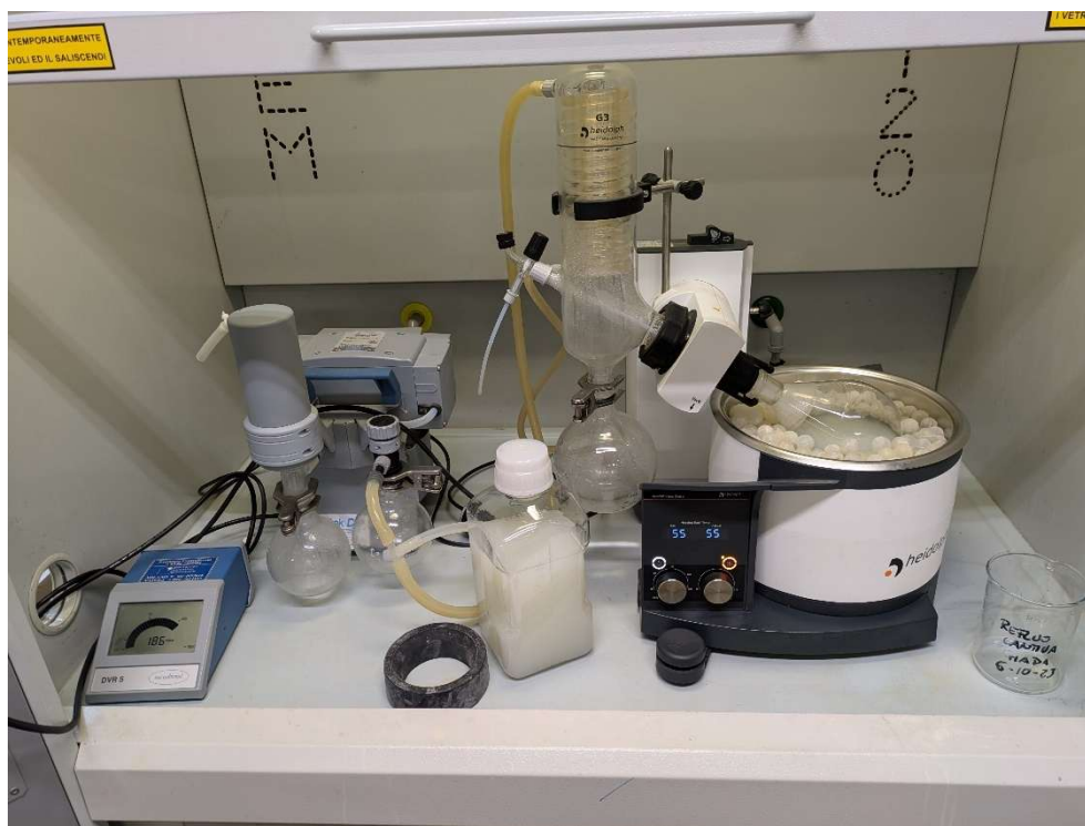
Figure 2.4: Experimental apparatus used for batch distillation in the laboratory.
