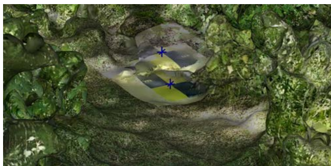
Figure 13. Example of the ambiguity created during the reconstruction of a few target points positioned in areas completely vegetated. The blue marker indicates the ambiguity of the target center.
