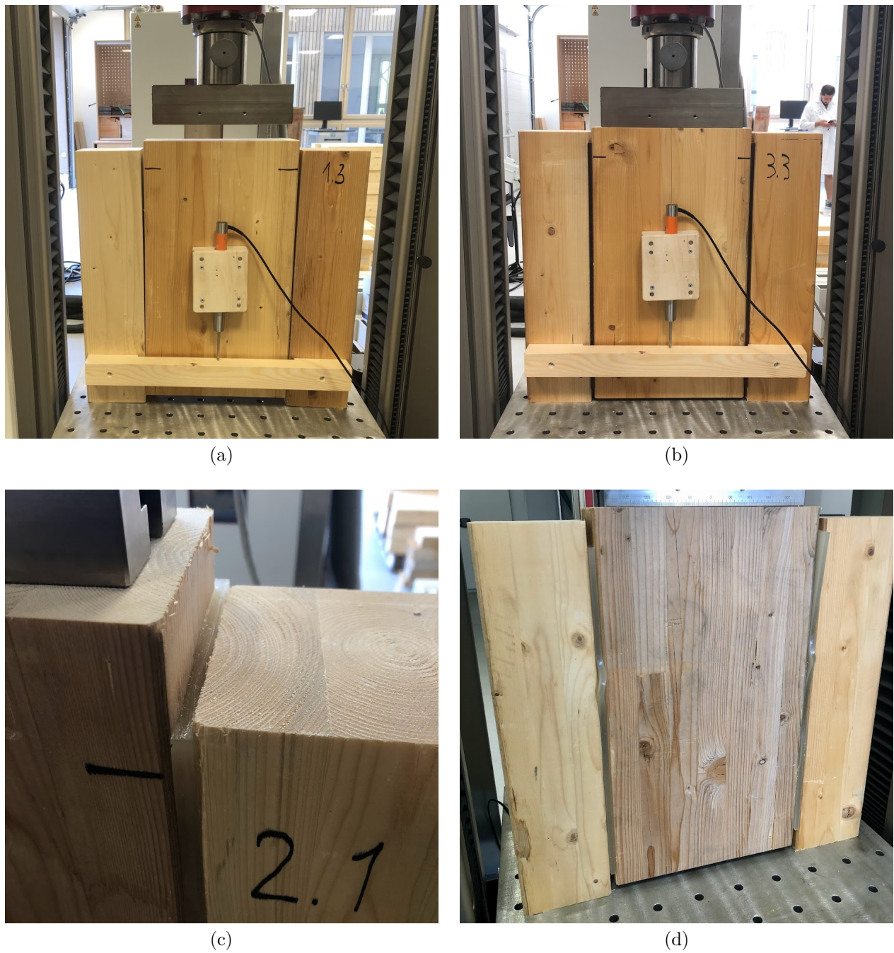
Figure 3.11: Timber-to-timber failure modes.
