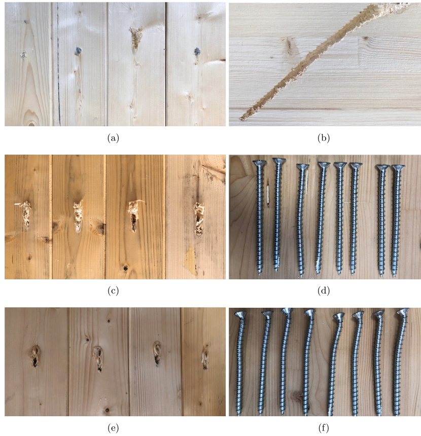
Fig. 5. Failure modes: (a) Screw and withdrawal with one hinge (b) Withdrawal with one hinge (c, d) Withdrawal (e, f) Double hinges.
