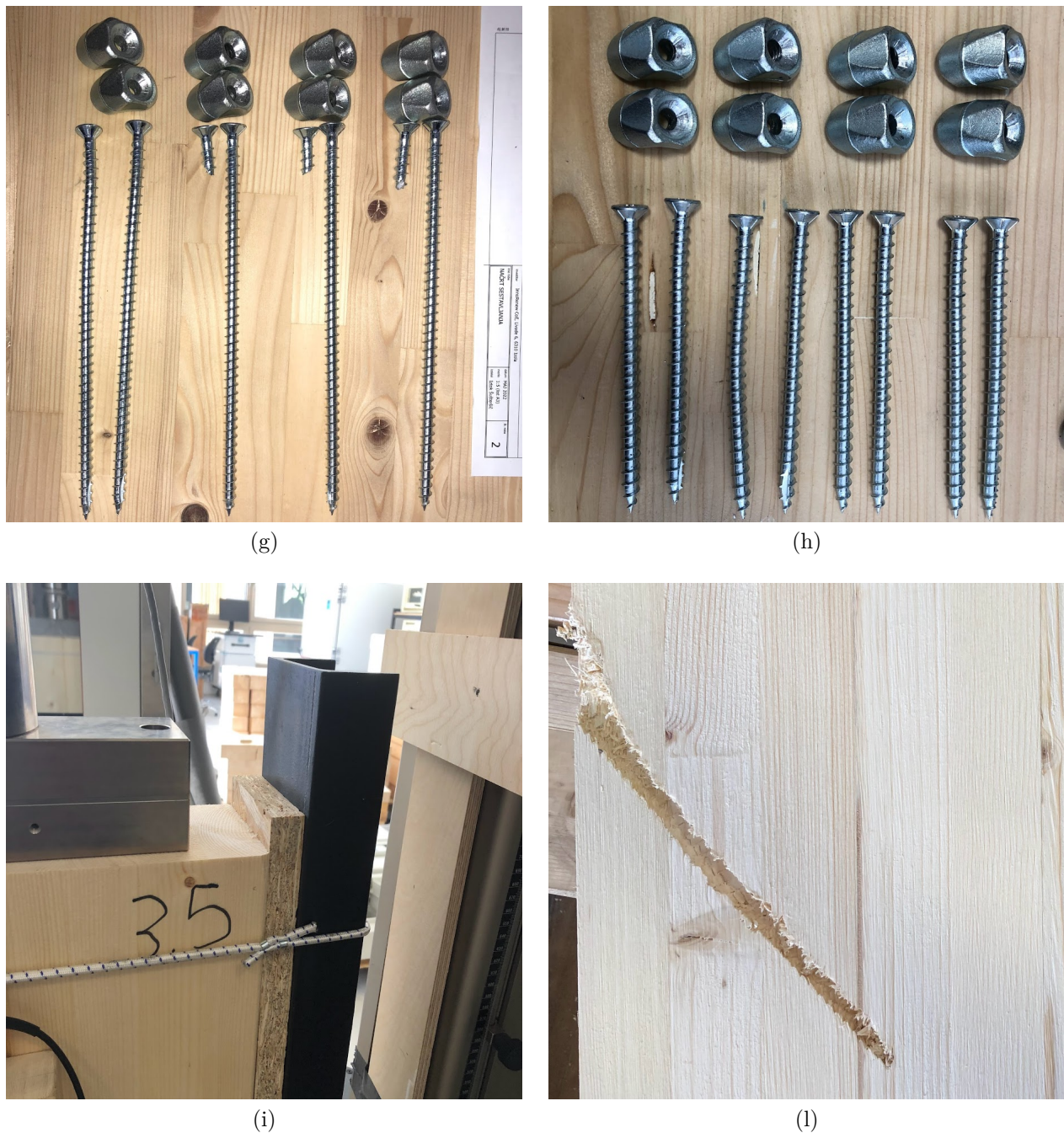
Figure 3.17: Timber-to-steel failure modes.
