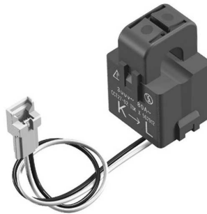
Figure 9.1: Current transformer sensor TDK CCT27-02.
