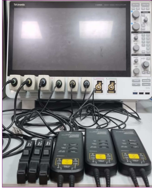
Figure 8.4: Tektronix 5 series MSO oscilloscope used in the experimental setup.
