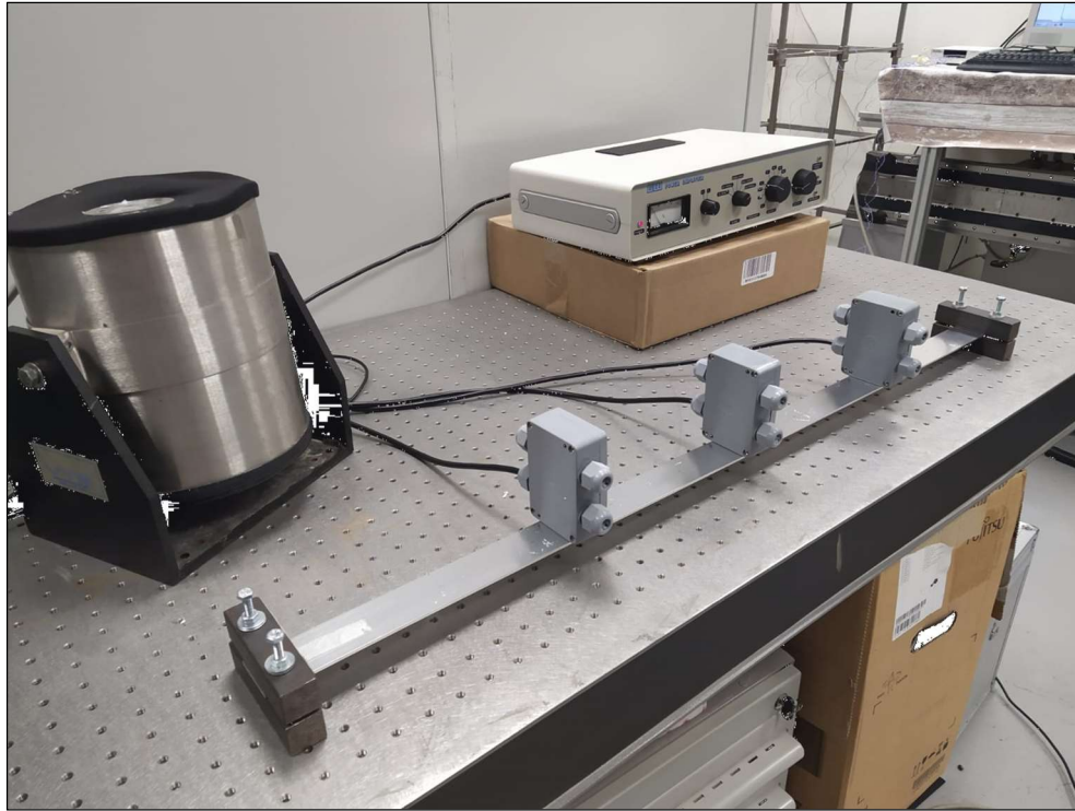
Figure 23: Metal bar excited by white noise.
