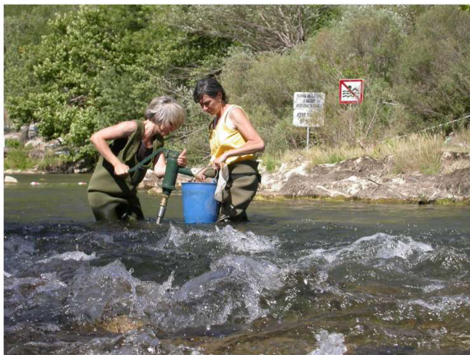
Figure 2. Sampling the hyporheic zone of the Hérault River with the Bou-Rouch pump (© V. Prié).
