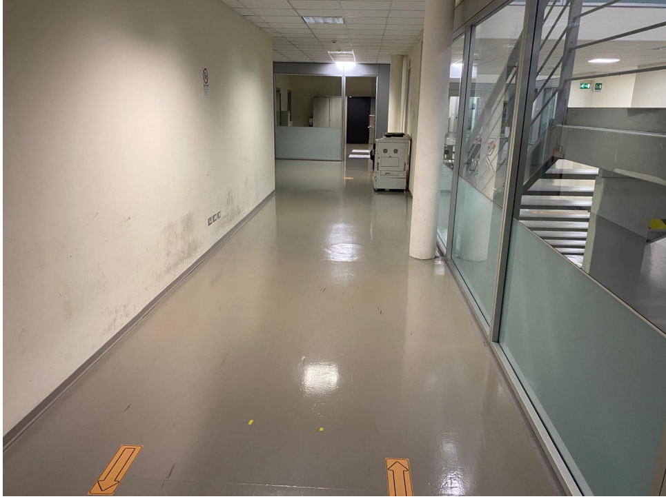
Figure 5.1: The experimental corridor environment. The uniform surfaces and lack of distinct geometric landmarks require precise scan-matching to prevent odometric drift.
