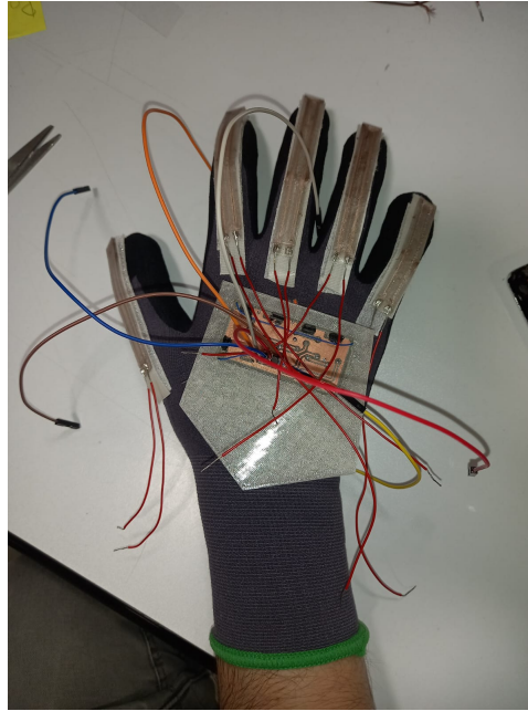
Figure 3.15. Smart glove with bending sensors.
