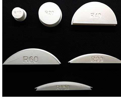
Figure 3.11. Curved samples for the strain gauge characterization.
