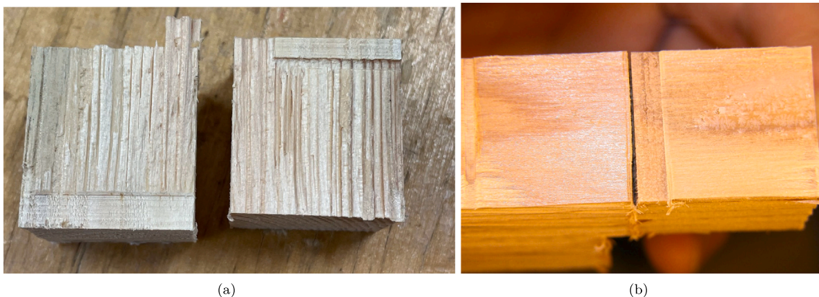
Fig. 3. View of a typical timber (a) and glue (b) failures.
