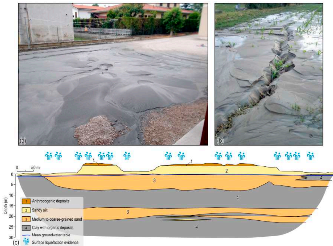
Figure 2. Liquefaction manifestations at the surface during the 2012 Emilia seismic sequence (modified from [31]). (a) Widespread liquefactions with series of sand-blows (Lat: 44.79317N Lon: 11.29129E).
