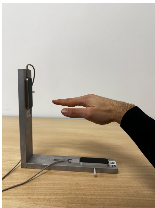
Figure 2. VG system while tracking the hand movements. The hand positioning system is united with the one of the VG.
