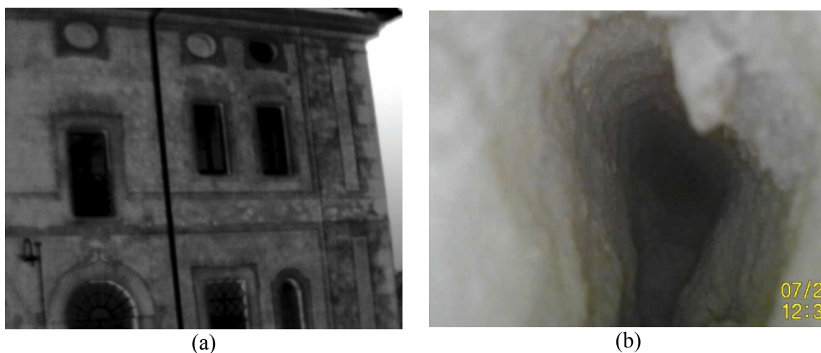
Figure 5. Masonry Class A3/I: infrared image (a), endoscopic image (b)
