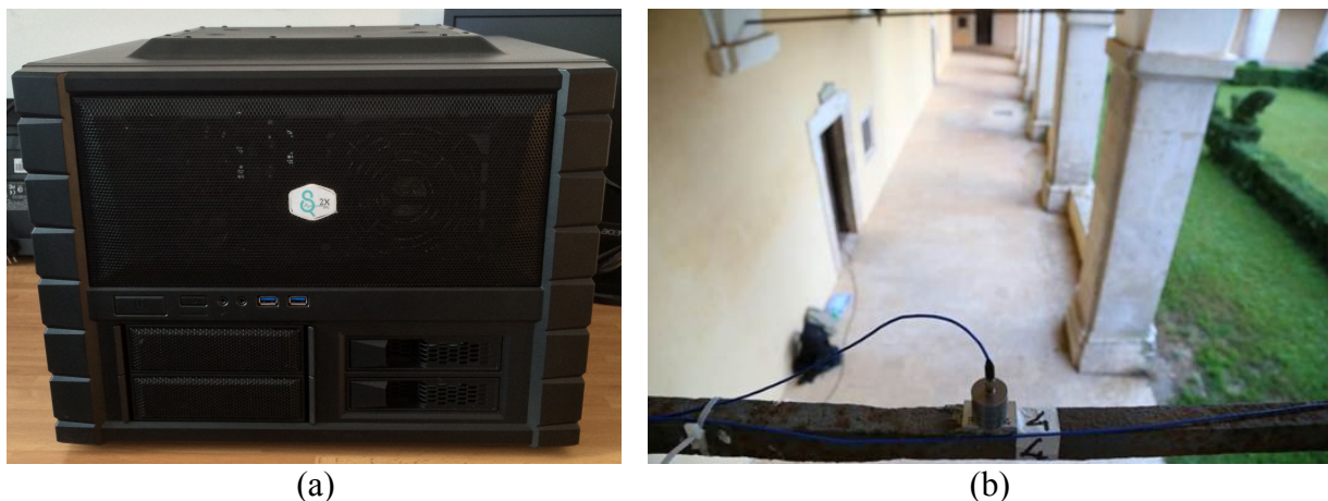
Figure 10. Vibration-based testing of tie-rods: measurement system (a), installed sensor (b)
