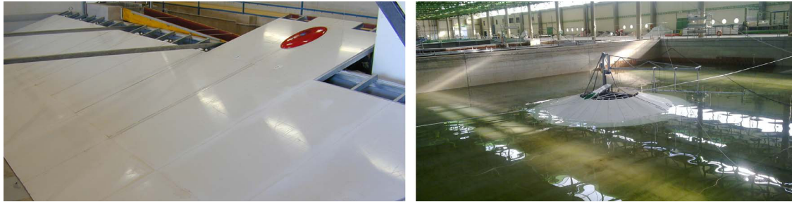
Fig. 1. Picture of the straight coast physical model (left) and of the conical island (right).
