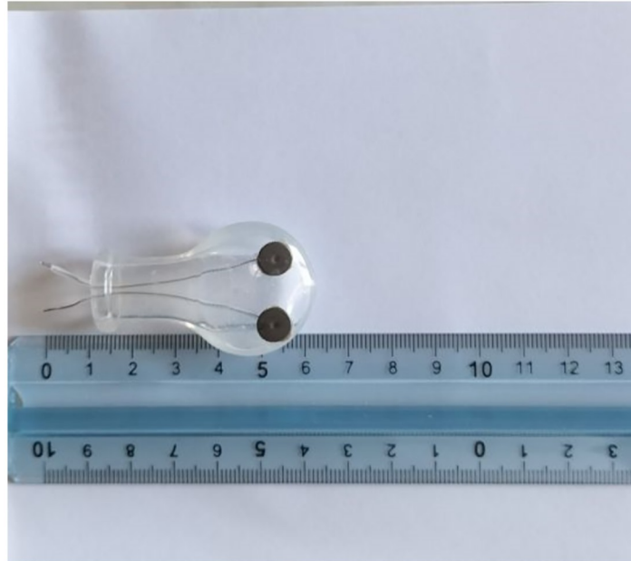
Fig 1. Pacifier with applied electrodes for electrical stimulation of the dorsal anterior surface of the tongue.
