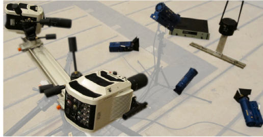
Fig. 2. The setup of the experimental measurement. From left to right: the two cameras, four spotlights, the sample clamped to the floor and connected to the shaker, and the signal amplifier.
