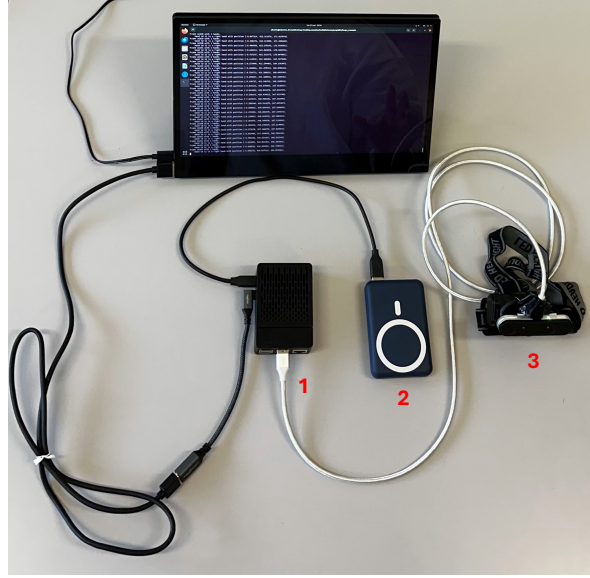
Figure 5.4: System embodiment: (1) the RP enclosed in its case, (2) the power bank, (3) the LMC inside the head-mounted support. The presence of the monitor, not used in the final embodiment, is necessary during system calibration to set the values of the parameters.
