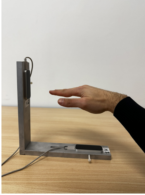
Figure 2.4: Assembly of the Virtual Glove system, consisting of two Leap Motion Controller (V1) sensors mounted orthogonally on an aluminum base. The image shows a potential user positioning the hand above the device, demonstrating the correct placement during task execution.
