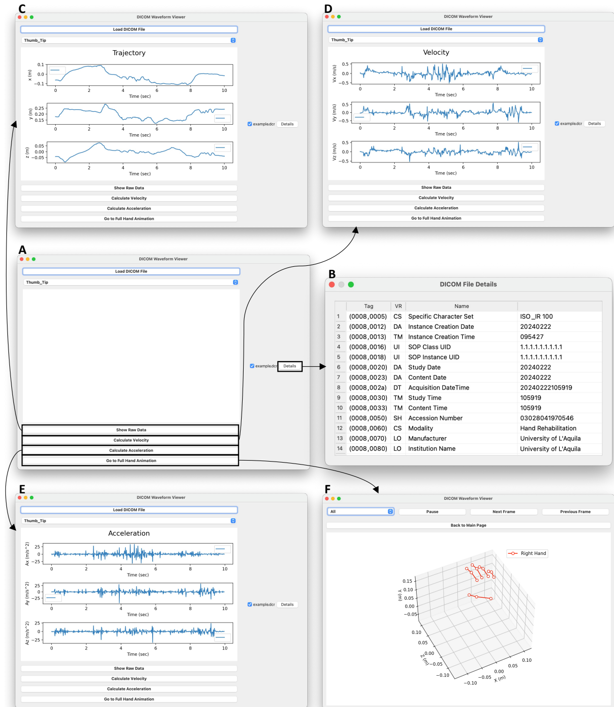
Figure 7.10: Viewer Interface for feature calculation and display: (A) Main Window for navigation through data and functions; (B) DICOM Field Window to show all fields, including TAG, VR, Name, and Value; (C) Trajectory feature components of a selected finger joint; (D) Velocity feature components calculated from the trajectory of the selected finger joint; (E) Acceleration feature components computed from the corresponding velocity; (F) Interactive Plot Window showing dynamic scatter plot animations of the hand as a whole or a specific finger.
