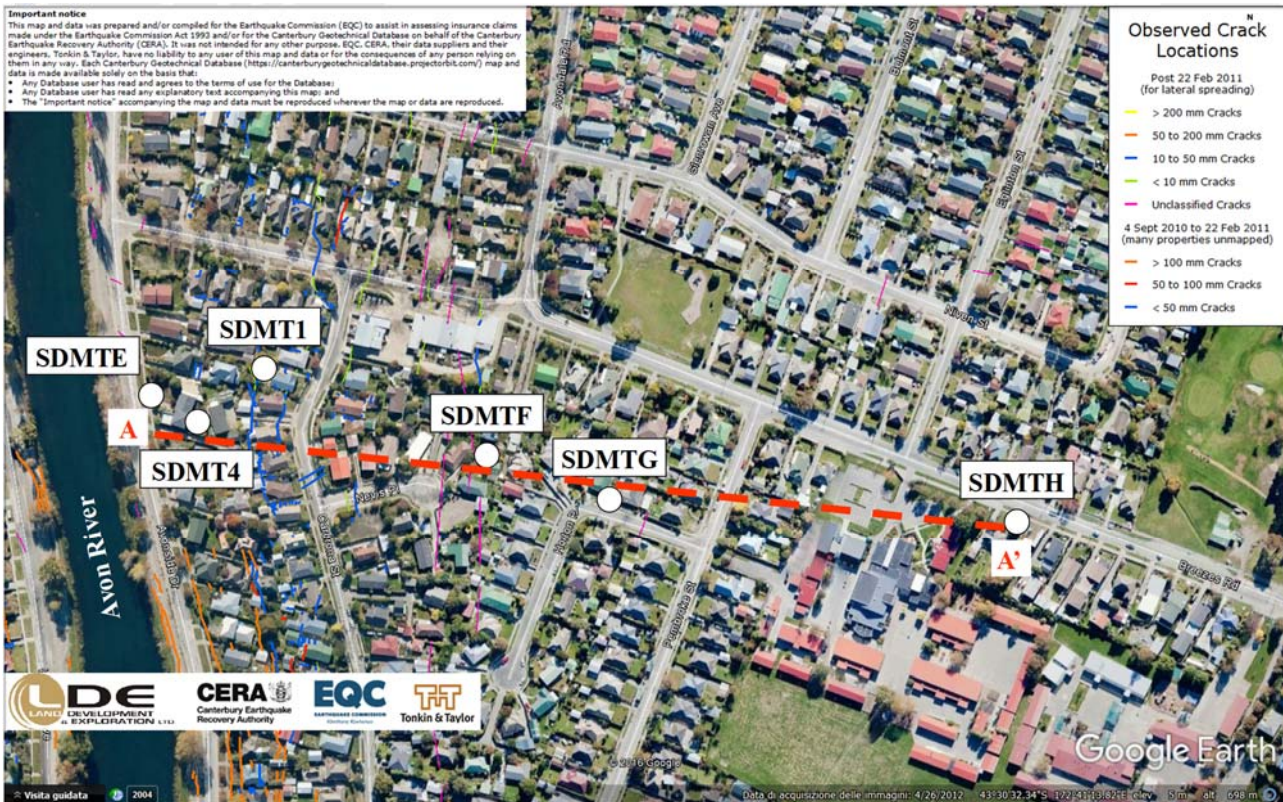
Fig. 1. Map of the observed cracks following the February 2011 seismic event in the area of study (Canterbury Geotechnical Database 2013). The map also shows the location of the SDMTs performed for the present study and the trace of the analyzed section.
