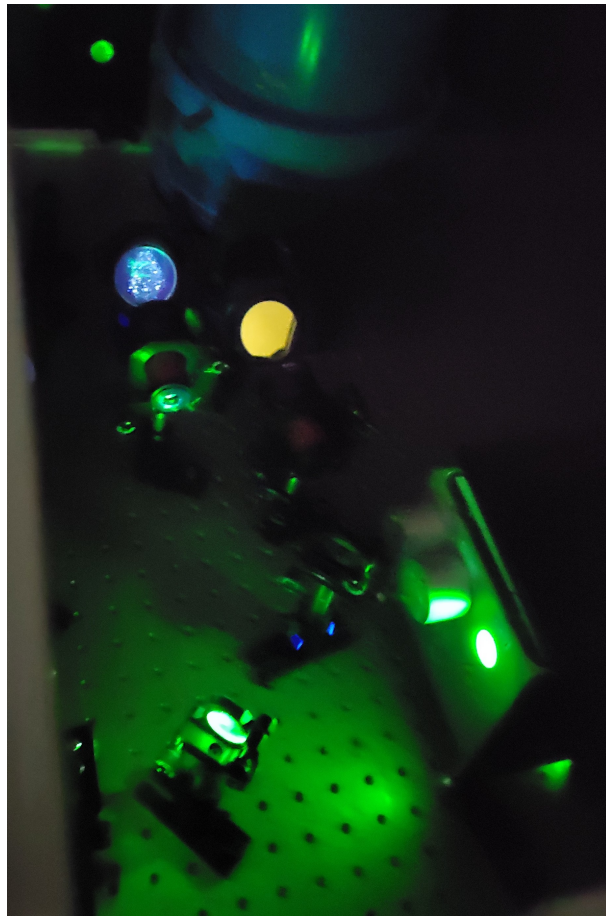
Figure C.7: Green contamination of the UV laser beam.
