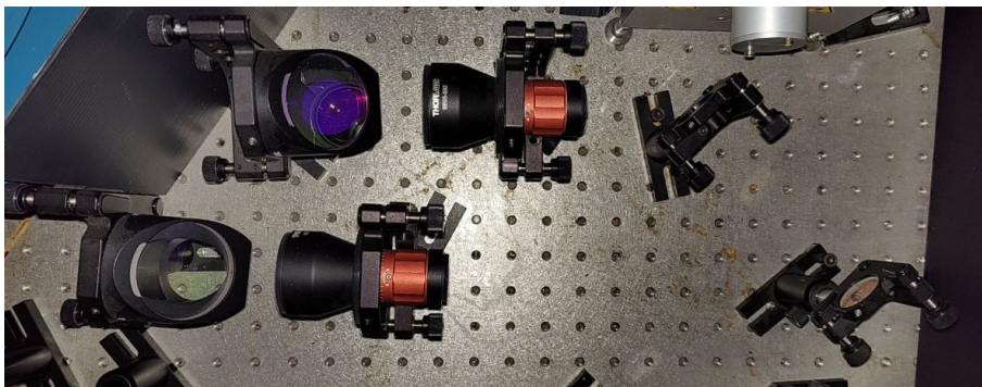
Figure 6.3: Transmission optics for laser beams at 355 nm (bottom) and 532 nm (top).
