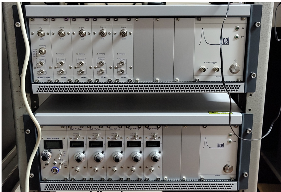
Figure 6.22: Licel Ethernet Controllers. On top there are the transient recorders while on bottom there are the power supplies of the detectors.
