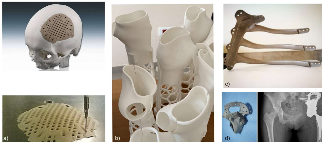
Fig. I. 17: Examples of biomedical implants and assistive devices manufactured by additive manufacturing using lattice and porous architectures: (a) patient-specific PEEK cranial implant featuring a perforated lattice structure for stiffness reduction and tissue integration [87]; (b) customized PA12 forearm orthoses produced by AM, exploiting lattice designs for weight reduction, ventilation, and wearer comfort; (c) 3D-printed titanium sternum implant fabricated by metal additive manufacturing, incorporating lattice regions to enhance osseointegration and mechanical compatibility; (d) pelvic implant manufactured by powder bed fusion using Ti-6Al-4V ELI alloy, illustrating the use of porous structures to promote bone ingrowth and reduce stress shielding.
