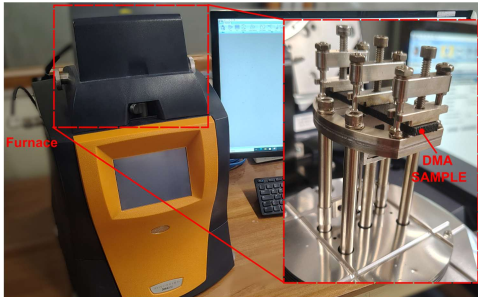
Fig. 2. 27: Dynamic Mechanical Analysis (DMA) experimental setup: DMA instrument equipped with an integrated furnace for temperature-controlled testing. In the magnified images of the internal of the furnace the double cantilever beam (DCB) fixture with the specimen clamped between three supports is presented, highlighting the loading configuration adopted for flexural DMA measurements.
