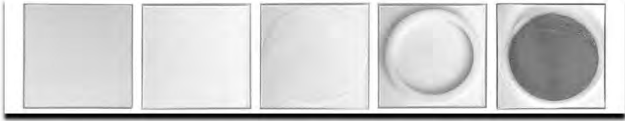
Figure 5. From the right: glass plate (GP), GP and filter paper plate (GFP), GFP and non-woven tissue (GFPT), GFPT and plastic ring (GFPTR), GFPTR with the fresh mortar placed.
