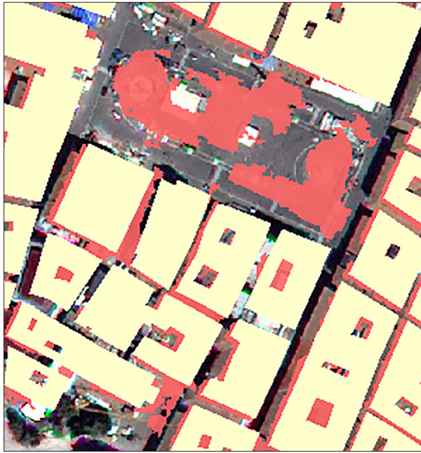
Figure 14 - Classification mistakes; the algorithms (red color) classify some paved areas as buildings not present in CTR buildings (yellow color).
