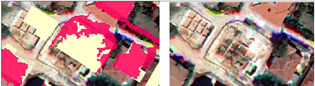
Figure 15 - Buildings collapsed and not identified by classification algorithms (red color)but reported on cartography (yellow color).
