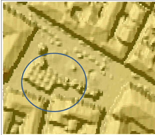
Figure 10 - GRID from LIDAR points used where mobile obstacles are evident ( http://www.pcn.minambiente.it/GN ).
