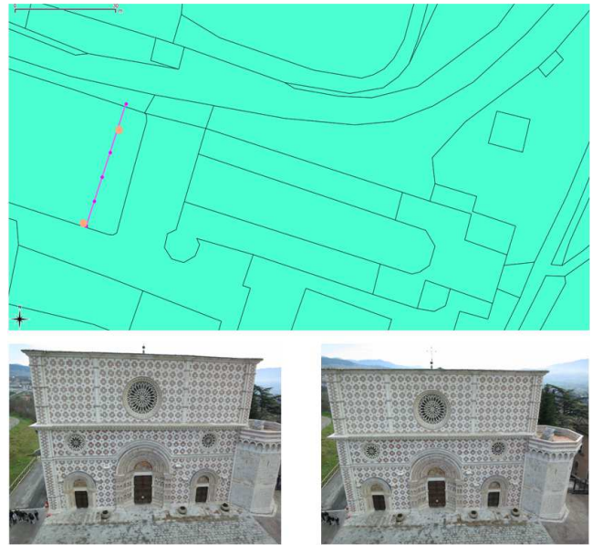
Figure 9. The stereopairs that have nearly the same geometry planned by the software
