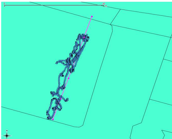
Figure 8. Comparison between the flight plan calculated by the software UP23d with that conducted by the UAV pilot
