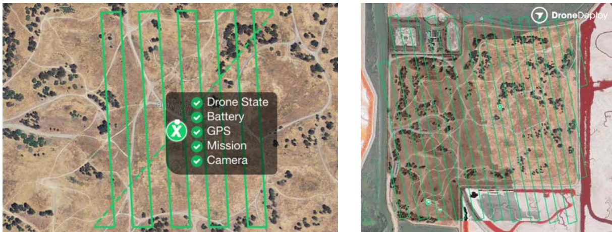
Fig. 2: Selection of the area to survey and of flight parameters (on the left), drone takeoff checklist (on the right) (Dronedeploy) drawn from: https://geosensornetworks.wordpress.com/2015/03/31/mobile-mapping-with-dronedeploy/ .
