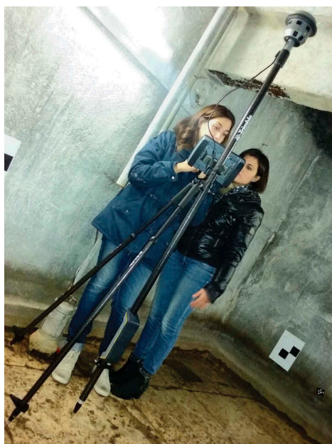
Figure 2. The Trimble V10 terrestrial imaging system: configuration for integration with total stations; on the right the visual field generated by the disposition of the cameras.
