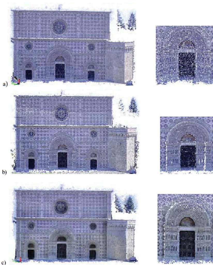
Figure 9. Point clouds following the compensation of automatic TPs: (a) from the survey at 60 m; (b) from the integration of the surveys at 60 and 40 m; (c) from the integration of the surveys at 60, 40 and 20 m.
