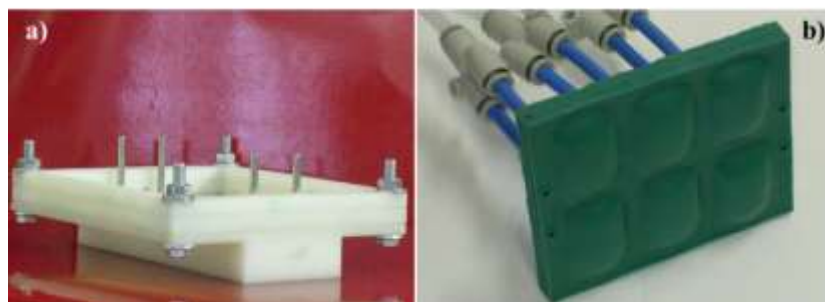
Figure 3 Prototyping of the actuator: a) the casting mold; b) the final prototype
