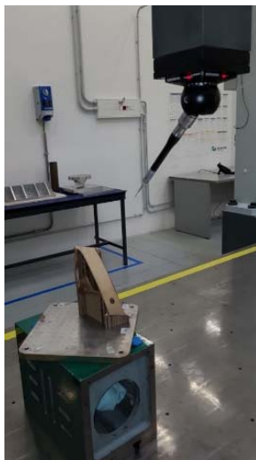
Fig. 6. CMM machine for measuring the component's surface
