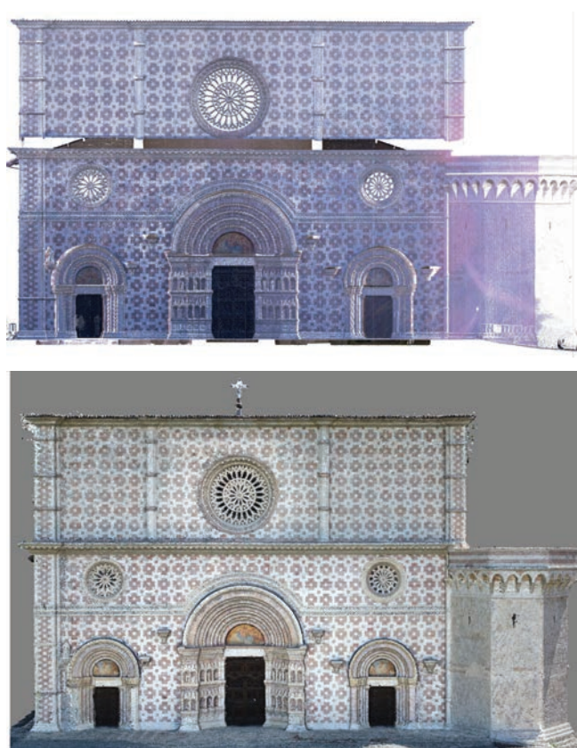
Figure 3. Comparison between the point cloud acquired by laser scanner to the left and by drone to the right.
