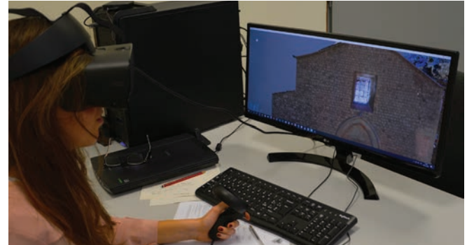
Figure 9. Navigation of the point cloud of St. Maria ad Cryptas through the use of a VR viewer and Scene software.
