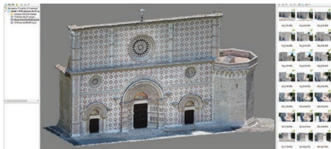
Figure 2. Facade of the Basilica of Collemaggio. View of the point cloud inside the Agisoft software.
