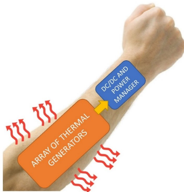
Figure 4.16 Block scheme of the proposed energy harvesting system. It is made on a printed circuit board with an array of thermoelectric generators placed on the front forearm of the user, a DC/DC converter and power manager unit [206].
