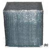
Figure 2. Comparison between two cubes based on the same nominal geometry and manufactured using a different acceleration value.
