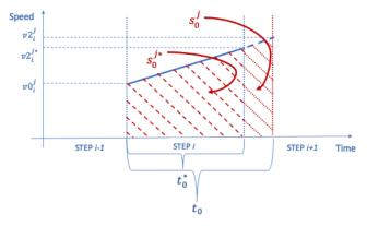
Figure 9. Insufficient distance for acceleration; new end speed.
