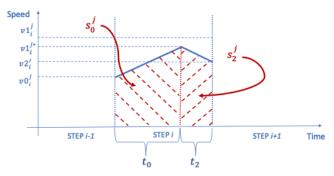
Figure 11. Nominal speed not reached. Sufficient space for accelerating and decelerating.
