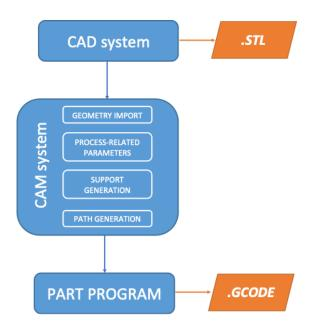
Figure 3. Automatic programming for generating the part program.
