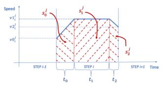
Figure 8. Nominal speed reached during step i-th.
