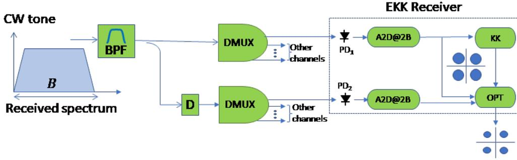
**Fig. 1.** The proposed EKK scheme. The received signal is split into two replicas, one of which is dispersed, so as to decorrelate the intensity patterns. The KK is used as initial condition for the algorithm.
