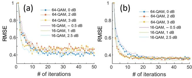
**Fig. 2.** The root-mean-square error of the recovered symbols as a function of the number of optimization iterations. Legends show modulation format and CSNR value. RMSE values are normalized to the result without optimization. (a) effective OSNR of 22 dB. (b) effective OSNR of 31 dB.
