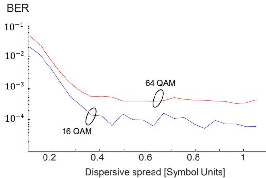
**Fig. 5.** BER vs. the dispersion of the dispersive module placed in the lower arm in the receiver in Fig. 1. The dispersive effect is quantified in terms of the dispersive spread of the signal in symbol units  $\beta''LB^2$ . The curves are plotted for CSPR= 3 dB and for an effective OSNR of 25 dB without fiber nonlinearity.
