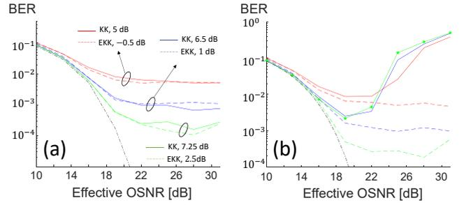
**Fig. 3.** BER vs. Effective OSNR for 16 QAM signal modulation in the cases of linear (a) and nonlinear (b) propagation. The dashed and solid curves correspond to EKK and KK, respectively. The legends in (a) show the CSNR in each of the cases and they apply also to plot (b). The dash-dotted curve is the theoretical curve of ideal coherent detection in back to back.
