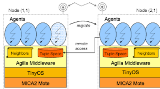
Figure 4.1: Agilla MW architecture
