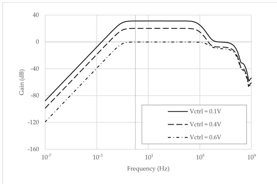
**Figure 8.** AC performances of the amplifier at various gain levels.
