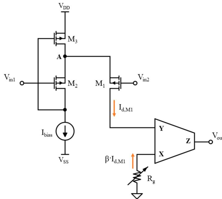
Figure 4. Mixed circuit and block scheme of the proposed DFVF-VCII-based amplifier.
