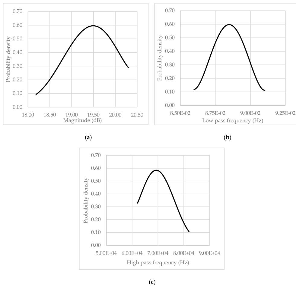
**Figure 12.** Statistical distribution of (a) the output voltage, (b) the lower cutoff frequency, (c) the higher cutoff frequency, evaluated under random PVT conditions.
