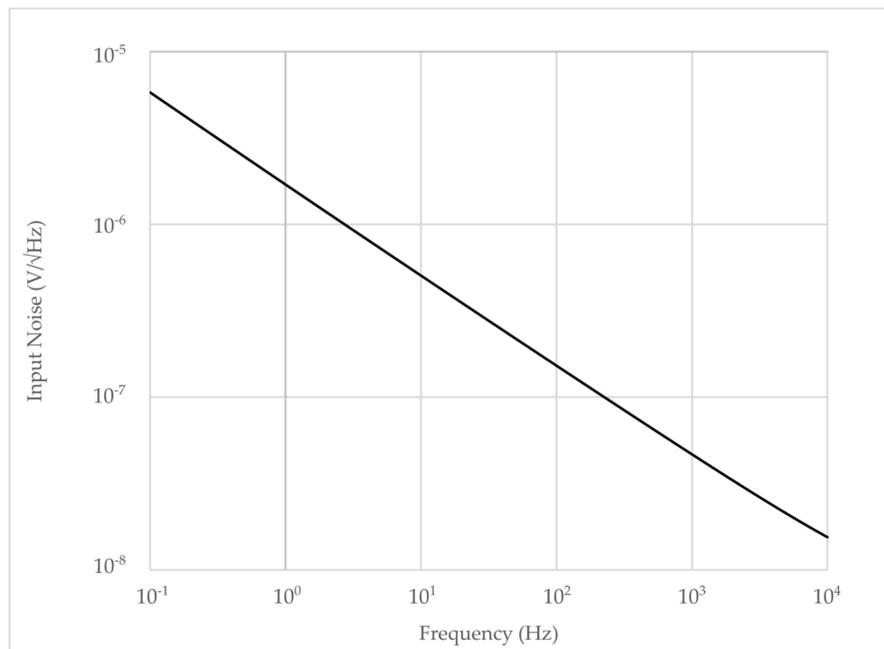
**Figure 10.** Input-referred noise performance of the amplifier.
