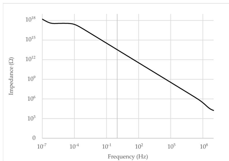
**Figure 11.** Input impedance of the proposed amplifier.
