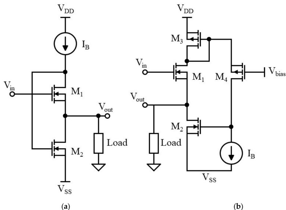
**Figure 1.** FVF structures: (a) standard NMOS FVF, (b) class AB FVF.
