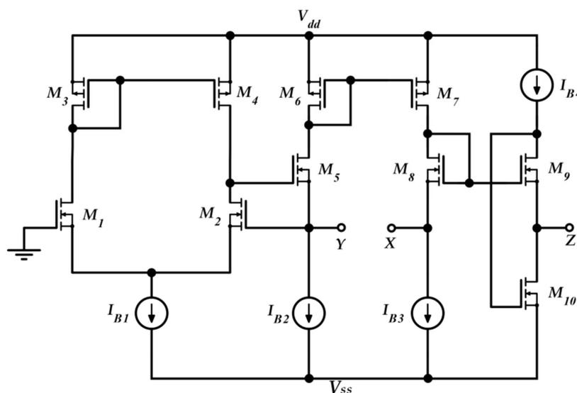
Figure 3. Transistor level implementation of the VCII+ used in this work.
