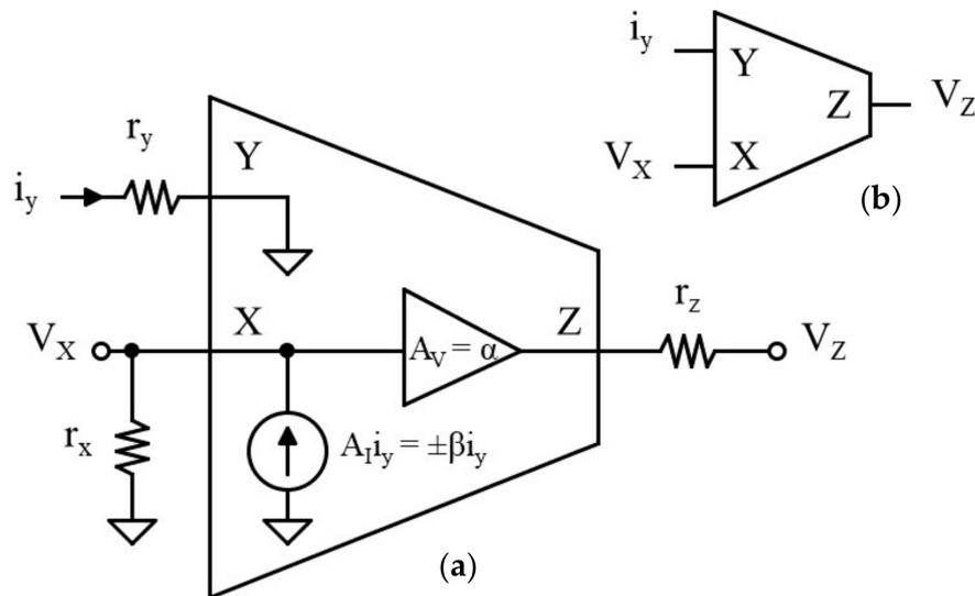
Figure 2. (a) Internal block structure of the VCII; (b) VCII device symbol.
