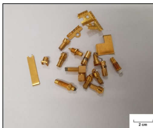
Figure 3. Third sample of connector and plated with the completely gold-plated surface.
