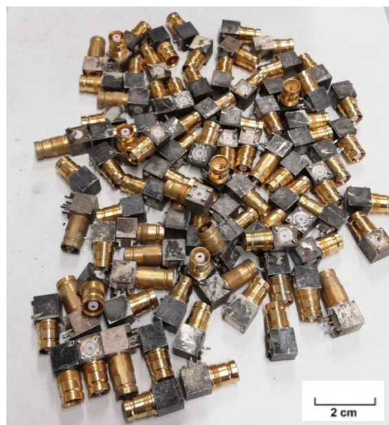
Figure 1. First sample of connectors with partial gold-plated surface.
