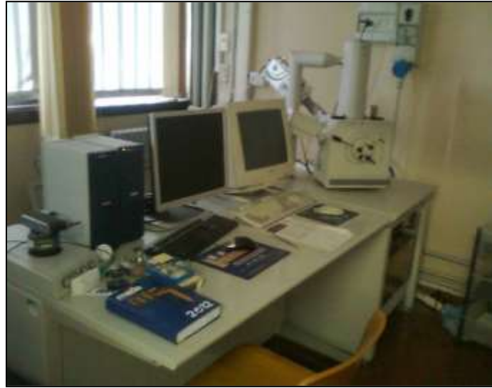
Figure 3.10: Philips XL30 CP Scanning Electron Microscope (SEM) equipped with an Energy Dispersive Spectrometer (EDS)
